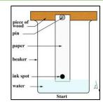
Different colours contain different mixtures of inks. The different inks move at different speeds up the paper. This is because of different solubility.
